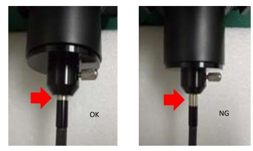
9.2.3 Failure of control box operation: Please ensure that the control box connector is properly installed and connected to the Hyper E640 lighting fixture.
