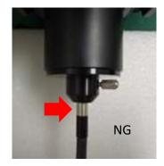
9.2.3 Control box operation failure: Please ensure that the controllor connector is securely connected to the Hyper E740 illuminator.
